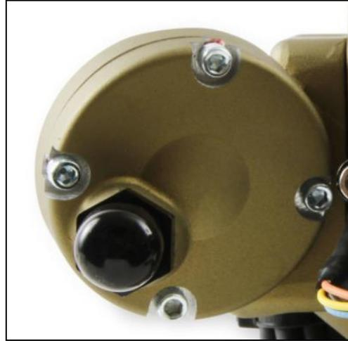
2. Remove the return line from the AN fitting on the cover (if applicable).
